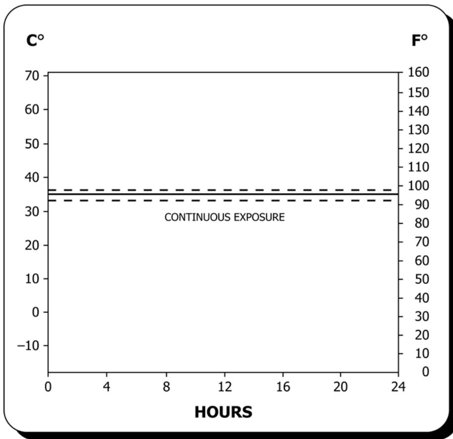
NOTE 1—Dashed chart lines indicate temperature tolerance limits.
