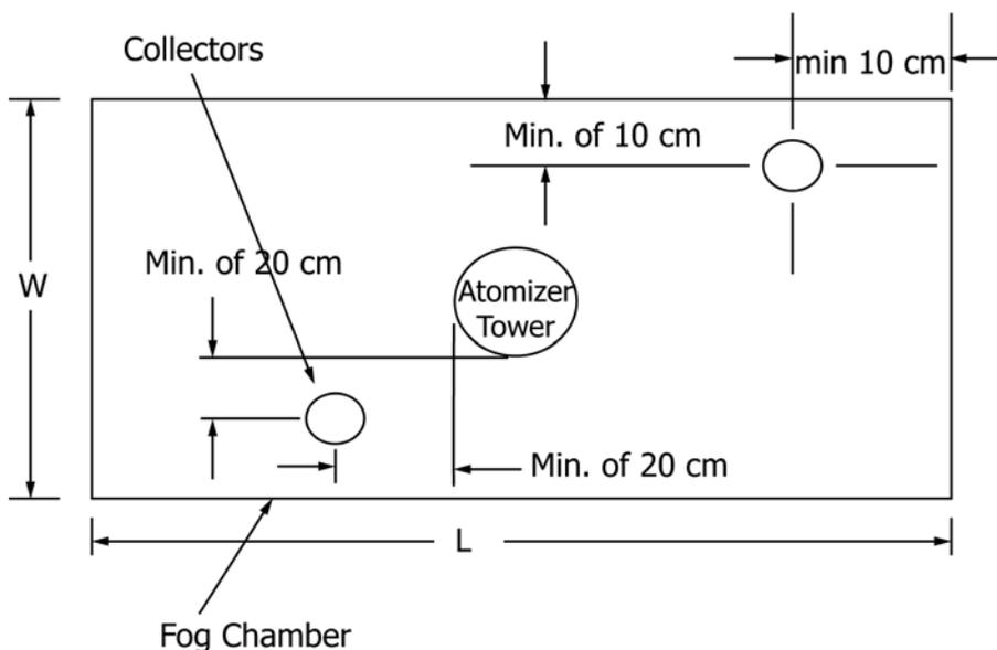
NOTE 1—This figure shows a typical fog collector arrangement for a single atomizer tower cabinet. The same fog collector arrangement is also applicable for multiple atomizer tower and horizontal ("T" type) atomizer tower cabinet constructions as well.
